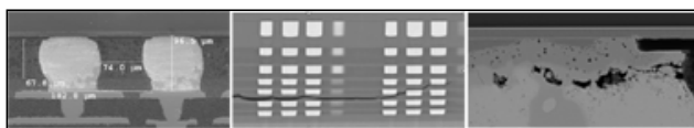
Figure 2: Solder fatigue, low-k dielectric cracking and electromigration voiding are the three main failure mechanisms in high performance flip-chip interconnects
