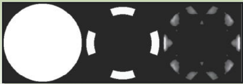
1. Examples of design targets used in the creation of DOEs for the semiconductor industry include (left to right) conventional illumination, quadrupole illumination and a complex freeform illumination. (Source: Mentor Graphics)
