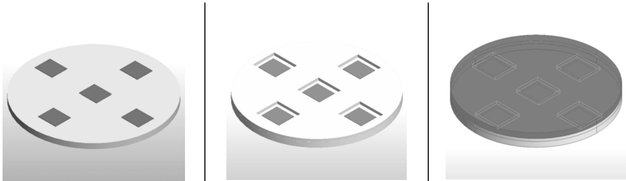
Fig. 1 Formation of a wafer level cavity package. Left - the device wafer containing five image sensors. Middle - application of the seal material to form a picture frame around the perimeter of each die. Right - attachment of a lid material to seal the cavity over each die with an air space between the device wafer and the cover glass. Singulation frees the packaged die from the wafer. Source: Tessera.
